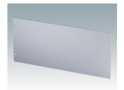
M6019050 Plaque avant 5Ux19" Aluminium Anodisé mat 482,6x3x221,45mm
